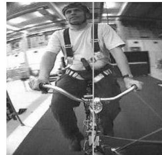
Figure 13. SCREEN-SHOT DIRECTLY AFTER A PERTURBATION (LATERAL FORCE APPLIED FROM THE RIDER'S RIGHT BY A ROPE AT THE SADDLE TUBE) AT 5 KM/H. VERTICAL GREY LINE INDICATES THE BICYCLE MIDPLANE. NOTE THE LATERAL RIGHT KNEE MOTION AND STEERING ACTION AND THE SMALL UPPER BODY LEAN ACTION.
