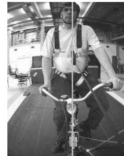
Figure 6. SCREEN-SHOT OF NORMAL PEDALING AT LOW SPEED (5 KM/H) SHOWING LARGE LATERAL (LEFT) KNEE MOTION AND (RIGHT) STEERING ACTION. THE GREY VERTICAL LINE INDICATES THE MIDPLANE OF THE BICYCLE. NOTE THAT THERE IS ALMOST NO UPPER BODY LEAN PRESENT.
