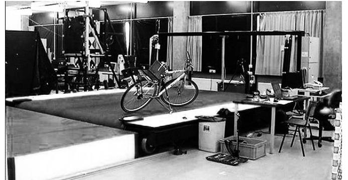
Figure 4. LARGE TREADMILL,  $3 \times 5$  M, MAX SPEED 35 KM/H, COUR-
