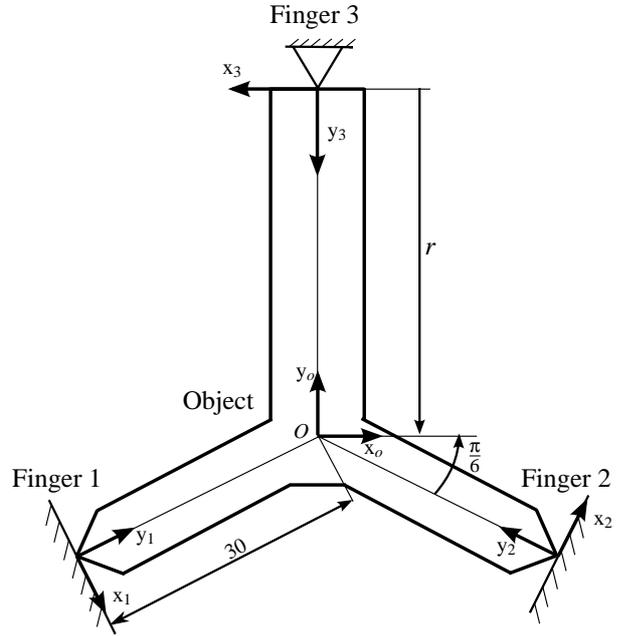
Figure 1. Grasp of a polygon by rigid fingers with zero (Finger 1 and 2) and infinite (Finger 3) curvature, adapted from [1]. Dimensions in [mm], [rad].
