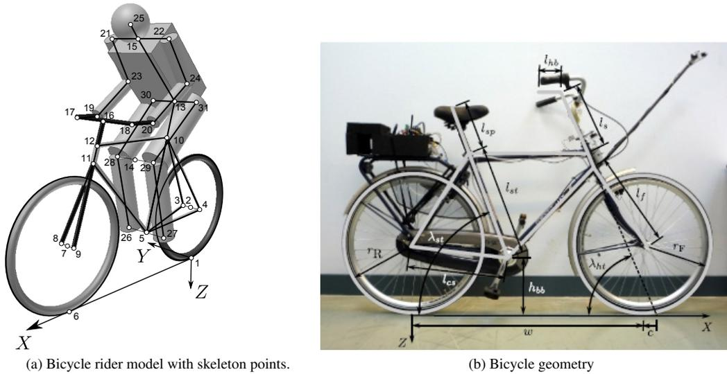
Figure 6: **a)** Bicycle rider model with skeleton points and **b)** bicycle geometry.
