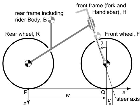
Figure 2: The bicycle model: four rigid bodies (rear wheel R, rear frame B, front handlebar assembly H, front wheel F) connected by three revolute joints (rear hub, steering axis, front hub), together with the coordinate system, and the degrees of freedom.
