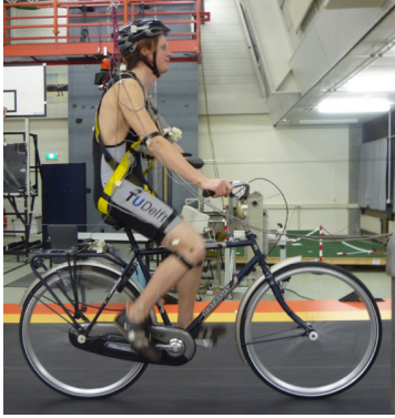
Figure 2. Rider posture on the Browser bicycle with an upright body and flexed arms on the handle bars. The degrees of freedom are the rear frame lean angle \phi , the upper body lean angle \theta , the steer angle \delta , and the forward speed v . The motion of the arms, connected to the handle bars, are passive, in the sense that they do not add any degrees of freedom to the system.
