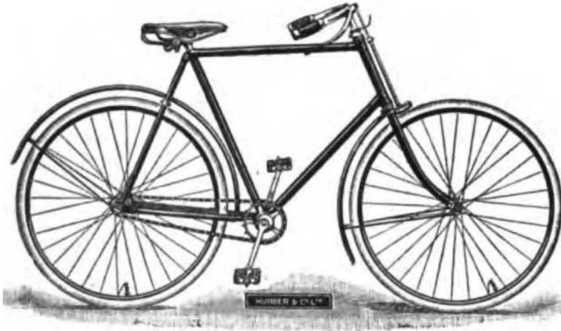
Figure 1. The safety bicycle, around 1890, from [9].
