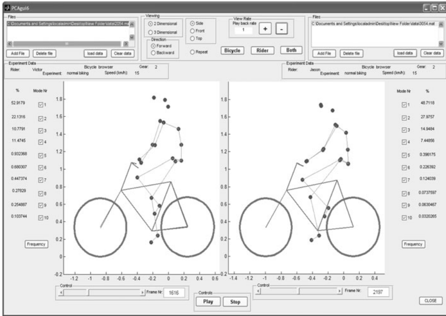
Fig. 6 Screen shot of the MATLAB graphical user interface (GUI) used to visualize principal components and compare between different components and trials
