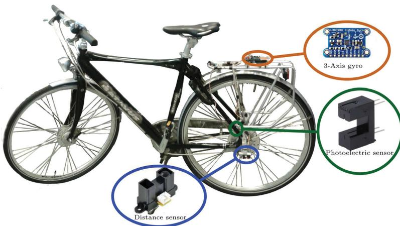
**Figure 6.** Instrumented bicycle, equipped with a photoelectric sensor to measure real wheel speed, and a three-axis angular rate sensor to estimate the roll angle. There are also two distance sensors for validation purposes.
