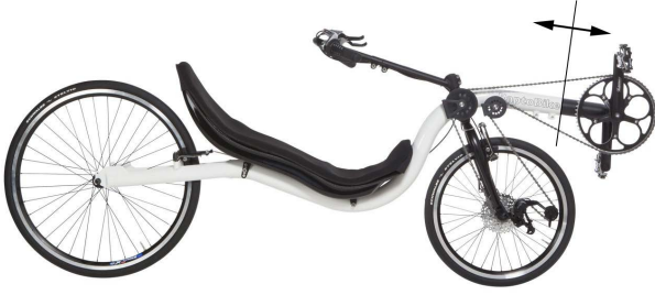
FIGURE 1. Raptobike Lowracer recumbent bicycle, existing design of a front drive recumbent bicycle. To accommodate variable size riders the drive train in front of the head tube can be extended, as indicated by the arrows.
