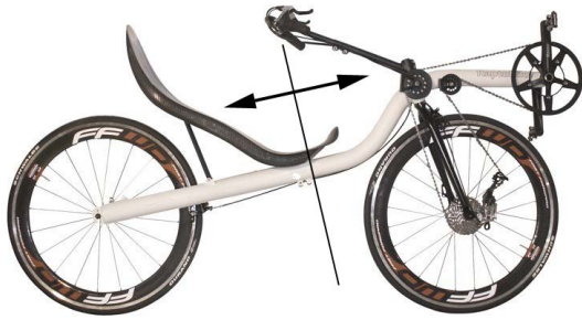
FIGURE 2. Raptobike Midracer recumbent bicycle, new design of a front drive recumbent bicycle. To accommodate variable size riders the rear frame tube between the rear axle and the head tube can be extended, as indicated by the arrows, keeping the drive train length unchanged. Shown is the short version.
