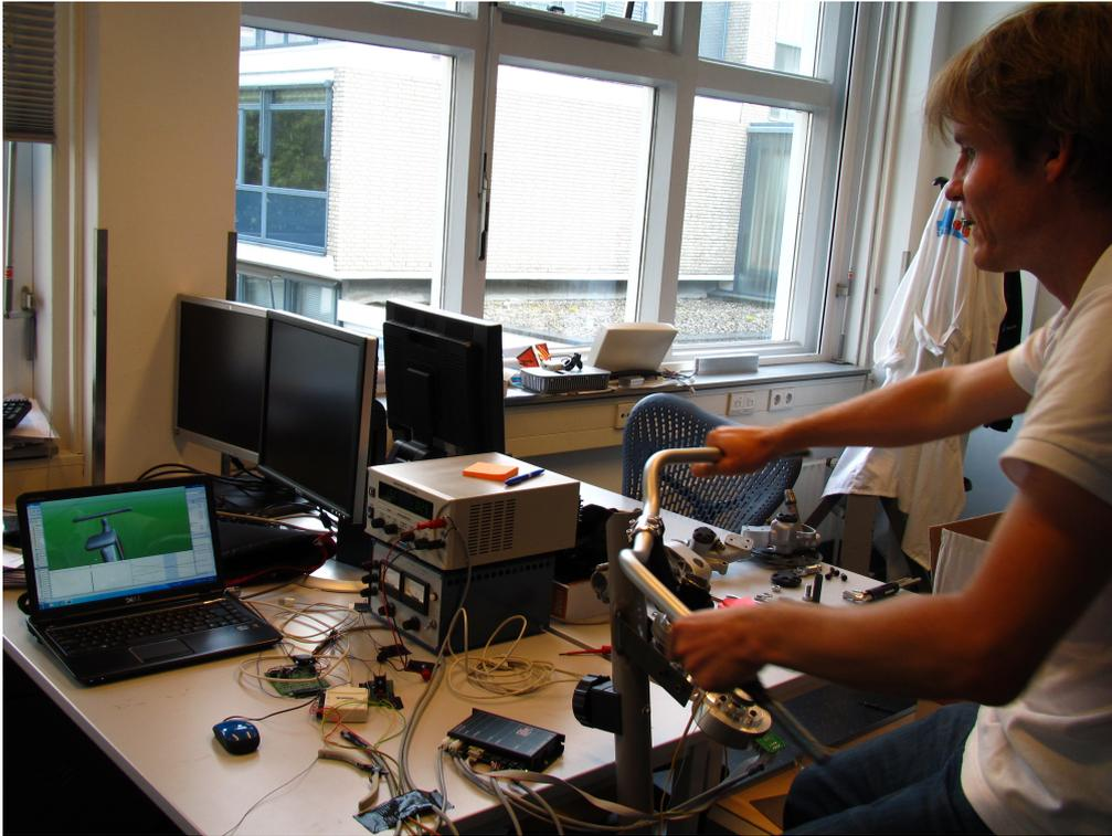
**Figure 3.** Experimental bicycle simulator setup with steering input device with haptic feedback and display with visual feedback.
