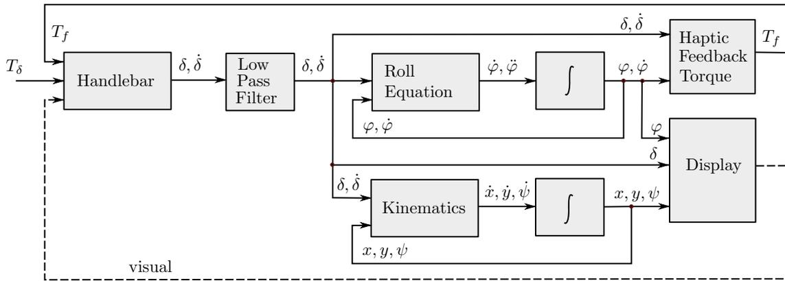
**Figure 4.** Block diagram of the bicycle simulator setup with the real handlebar dynamics, the measured and filtered steer angle  $\delta$  and steer rate  $\dot{\delta}$ , the computer model roll equation and kinematics, the generated haptic feedback torque on a visual display. The hardware for this system is shown in Figure 3.
