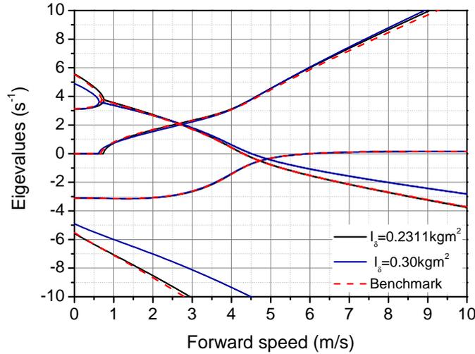
**Figure 2.** Eigenvalues of the benchmark bicycle in a forward speed range of  $0 < v < 10$  m/s, dashed red lines, compared with the eigenvalues of the bicycle simulator with two different mass moments of inertia  $I_\delta$ , an approximate value of  $0.3 \text{ kgm}^2$ , solid blue lines, and the value of  $I_\delta = \lambda_2 = 0.2311 \text{ kgm}^2$ , solid red lines. Note the striking similarity in eigenvalues between the benchmark and the simulator with  $I_\delta = \lambda_2$ .
