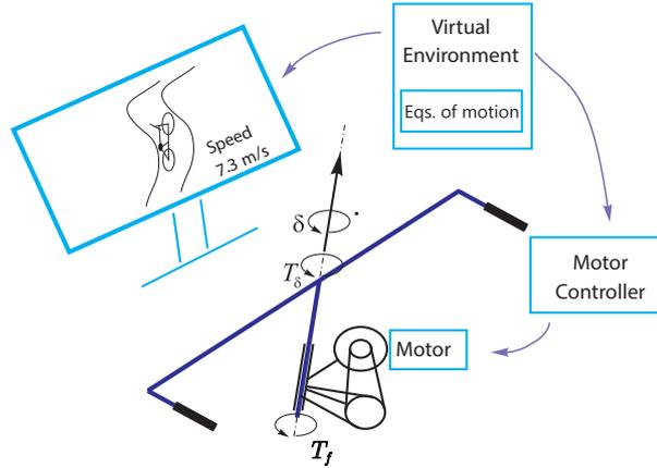
**Figure 1.** Scheme of bicycle simulator setup with haptic handlebar.  $T_f$  is the haptic feedback torque generated by the motor,  $T_\delta$  is the torque applied by the user,  $\delta$  is the degree of freedom of the system: the angle turned by the real handlebar
