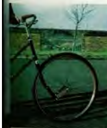
"UNRIDEABLE" BICYCLES. David Jones is seen here with three of his experimental machines, two of which turned out to be rideable after all. At top of this page is URB I, with its extra counter-rotating front wheel that tests the gyroscopic theories of bicycle stability. At left is URB III, whose reversed front forks give it great stability when pushed and released riderless. URB IV (immediately above) has its front wheel mounted ahead of the usual position and comes nearest to being "unrideable." —FIG. 1
