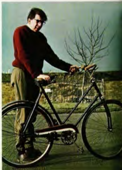
"UNRIDEABLE" BICYCLES. David Jones is seen here with three of his experimental machines, two of which turned out to be rideable after all. At top of this page is URB I, with its extra counter-rotating front wheel that tests the gyroscopic theories of bicycle stability. At left is URB III, whose reversed front forks give it great stability when pushed and released riderless. URB IV (immediately above) has its front wheel mounted ahead of the usual position and comes nearest to being "unrideable." —FIG. 1
