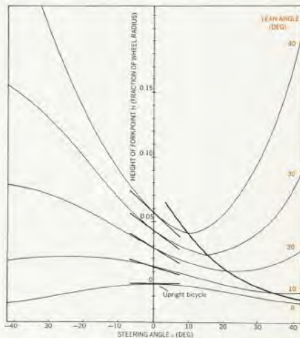
COMPUTERIZED BICYCLES. These data, from BICYC output, show that the minimal height of the forkpoint occurs nearer to the straight-ahead position for greater angles of lean. Note also that dH/d\alpha varies linearly with lean angle L for small L . Curves, computed for typical steering geometry (26-deg fork angle, 0.2 radii front projection), are vertically staggered for clarity.
