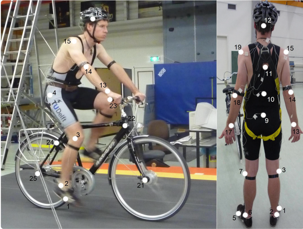
Figure 3.3: Bicycle and rider instrumented with active markers for motion capture while riding on a large treadmill
