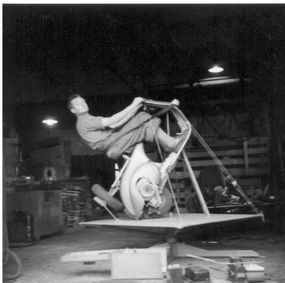
Figure 4.1: Test setup used by Döhning [35] to measure the moments of inertia of a motorcycle and rider. This photograph is a scan of the original which can be found in his thesis in the ETH Zurich repository.
