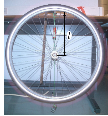
Figure 3. FRONT BICYCLE WHEEL MOUNTED IN A COMPOUND PENDULUM FROM [3].
