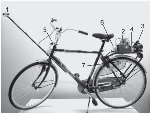
Figure 1. THE INSTRUMENTED BICYCLE WITH CAMERA BOOM AND VIDEO CAMERA LENS (1). ON THE REAR RACK THE MEASUREMENT COMPUTER (2), VIDEO CAMCORDER (3) AND BATTERY PACKS (4) ARE POSITIONED. MEASURED SIGNALS ARE THE STEER ANGLE AND STEER-RATE (5), REAR FRAME LEAN- AND YAW-RATE (6) AND FORWARD SPEED (7).
