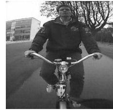
Figure 2. SCREEN-SHOT OF VIDEO MADE WITH THE BULLET CAMERA CONNECTED TO THE BICYCLE FRAME, FACING REARWARDS, SHOWING THE RIDER POSITION DURING NORMAL CYCLING.
