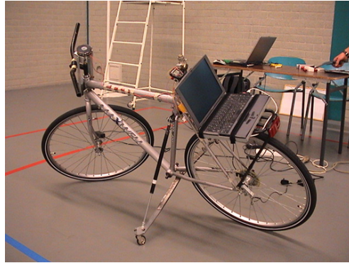
Figure 5.3: Instrumented bicycle from [81], with all the measurement equipment installed. Sensors are present for measuring the roll rate, yaw rate, steering angle, and rear wheel rotation. Data are collected via a USB connected data acquisition unit on the laptop computer, mounted on the rear rack.
