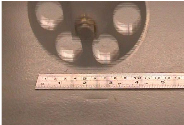
Figure 5.19: snapshot of the TU Delft sports hall nr. 2 floor directly after the wheel of the experimental TMS bicycle has been lifted up off the ground. The 2 cm wheel indent is clearly visible (5–7 cm) below the ruler.
