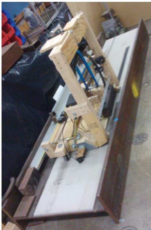
Figure 7. The test device on its final track: the self-levelling compound poured on the web of a large steel I-beam. The black strip of anti-skid tape can be seen along the right edge and the extruded aluminium strip along the left edge.
