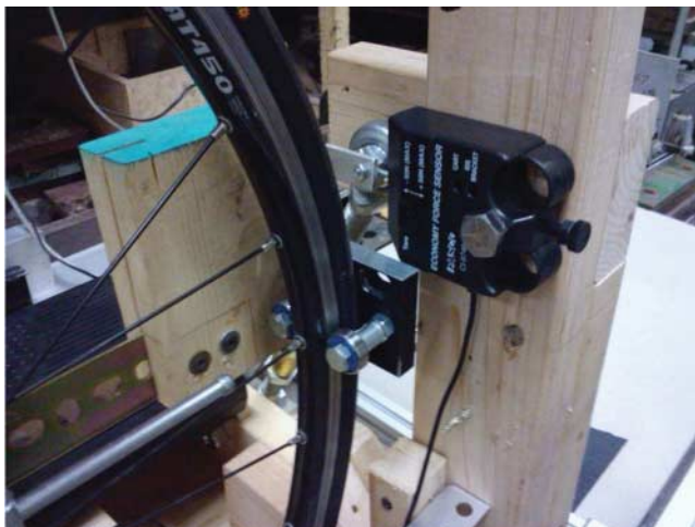
Figure 6. Mechanism to enforce wheel orientation and measure torque generated about the steering axis.
